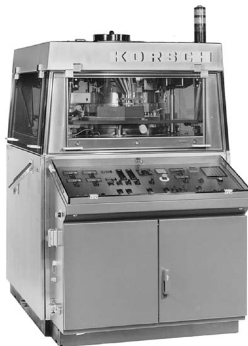
Fig. 22-11. Example of a production tablet press. (Courtesy of Korsch Tableting, Korsch AG, Berlin.)
