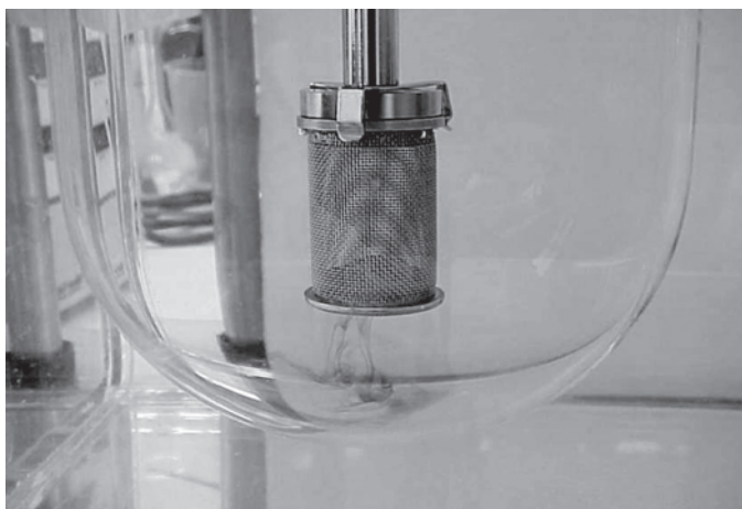
Basket apparatus No stirring
